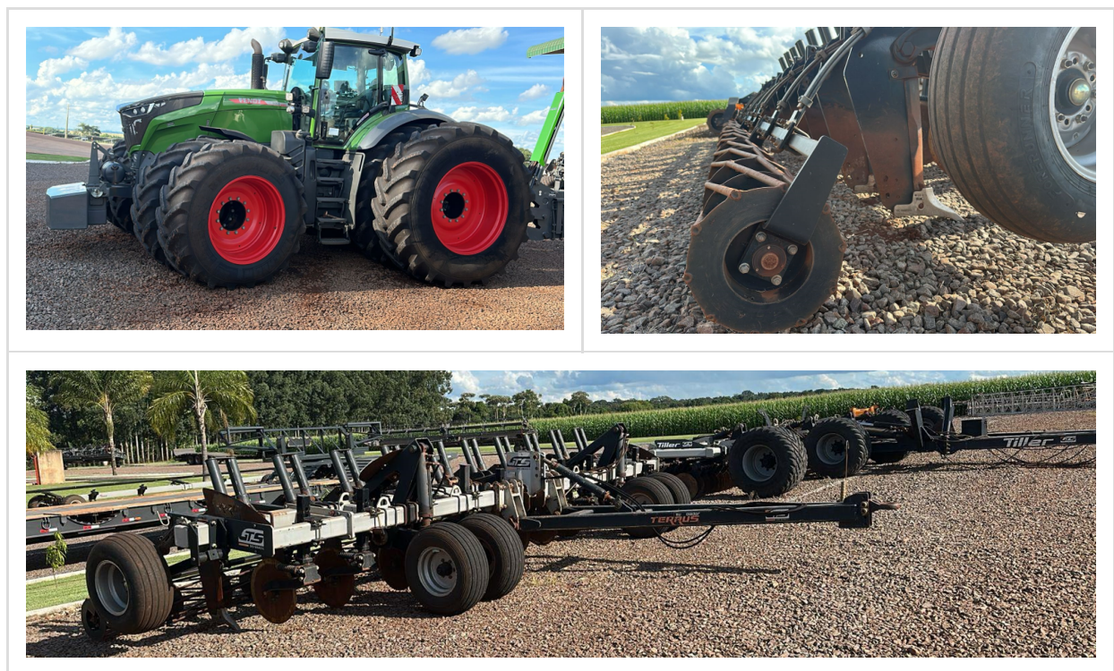
Figure 1. Equipment used: 517 hp Fendt 1050 Vario + 10-shank Terrus subsoiler, operating to a depth of 60 cm.
